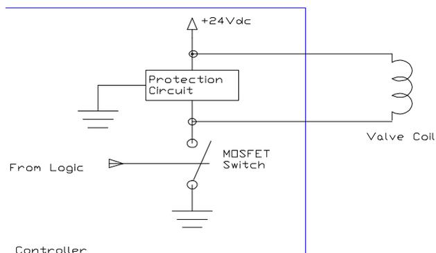
It should be noted that +24Vdc is supplied to one side of the valve coil at all times that the Controller is on. The other side of the coil will have 24V on it if the valve is off and approximately 0V if the valve is on. The +24Vdc line is normal if the voltage is between 22Vdc and 24Vdc.
