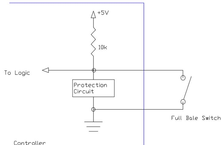
The baler is designed to complete its cycle and stop with the pressing fingers holding load onto the material in the hopper. There is sufficient internal leakage in the hydraulic system to allow the pressing fingers to creep up over time and possibly give a false full bale indication. To prevent this the Controller only monitors the full bale switch for 32 seconds after the pressing fingers stop in the down position.
